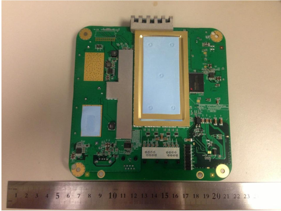
Photo 7- Main Board Back View
